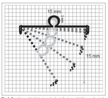
Fig. 1: Template used to fabricate and activate the transpalatal bars under study. Braz J Oral Sci. 9(1):16-19
