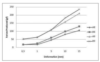
Fig. 3. Graph showing forces released by the bars for dislocations ranging from 0.5 to 15 mm.
