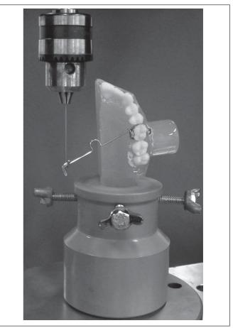
Fig. 2. Device used to attach the bars during the mechanical tests.
