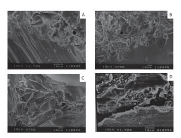
Fig. 1. SEM images of commercially pure titanium specimens with different ceramic materials used in study: Noritake Ti22 $^{\circ}$  (A), Triceran $^{\circ}$  (B), IPS $^{\circ}$  (C) and Noritake EX-3 $^{\circ}$  (D).
