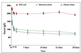
Fig. 2 - Force distribution (gF) of space closure materials over 28 days of evaluation.
