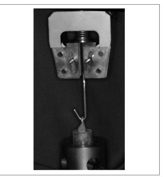
Fig. 2. Specimens subjected to tensile load at 180° in a universal testing machine.
