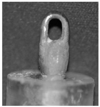
Fig. 1. Specimens embedded in acrylic resin before tensile strength testing in a universal testing machine.
