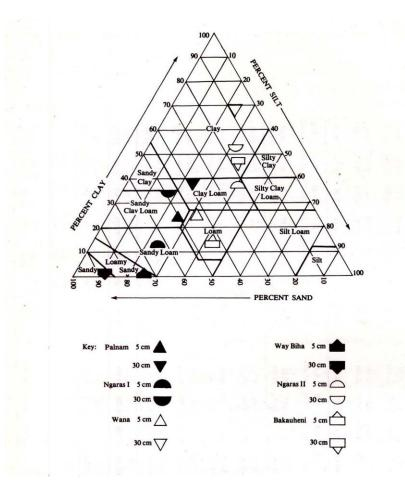
Figure 1. Soil texture triangle, showing position of soils listed on Table 2.
