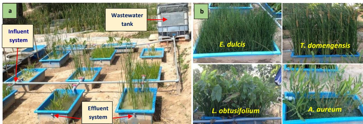
Figure 1 a) Experimental design with a treatment system; b) plant growth after 3-months handling
