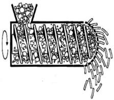
Fig. 1: Axial Screw feed extruder
