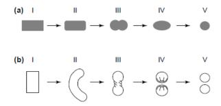
Fig. 8:Pellet-forming mechanism according to: (a) Rowe – I) Cylinder; II) Cylinder with rounded edges; III) Dumb-bell; IV) Ellipse; V) Sphere. (b) Baert – I) Cylinder; II) Rope; III) Dumb-bell; IV) Sphere with a cavity outside; V) Sphere.<sup>28</sup>
