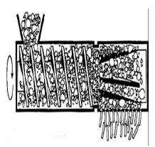
Fig. 2: Radial Screw feed extruder
