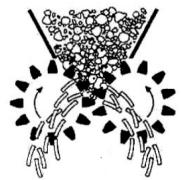
Fig. 6: Gear roll type
