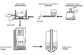
Fig. 9: Extrusion-spheronization process.
