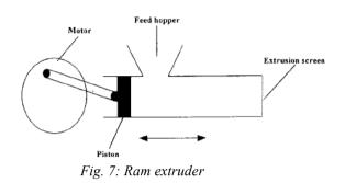
The extruded masses must have enough plasticity to deform, at the same time it must not adhere to other particles when rolled during spheronization process. This process mainly determines the final particle size of the pellets. The diameter of the extruder screen opening directly controls the diameter of the extrudate.<sup>24, 25</sup>
