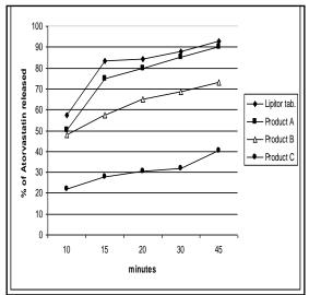
Figure 3 :dissolution profiles of some commercial products of Atorvastatin tablets; where product A ( Avas-20,MICRO Lab.India) was bioequivalent to Lipitor tablet ,however the product B (Atorvatin ,Alfaris Co.Syria) and product C (Atorvast 20,Avanzor,Syria) showed low dissolution .
