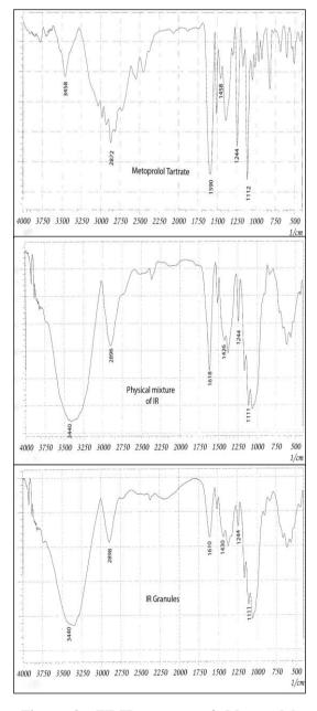
Figure 9: FT-IR spectra of Metoprolol, physical mixture and granules of the IR layer.
