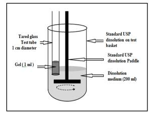
Figure (1): Modified USP XXIII in vitro dissolution testing apparatus
