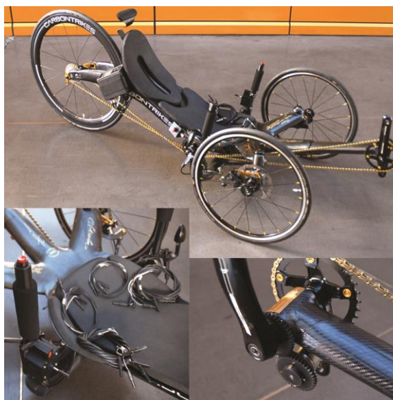
Fig 2. General view of the Tetratrike with details on the throttle, brake and encoder's gears. In the top figure, the stimulators are fixed on opposite sides of the frame behind the seat. In the left bottom angle is a handle with a red push button on top for an instantaneous stop of the stimulation, and a joystick with a display for changing the intensity of stimulation in discrete steps by a simple push of the joystick downwards. On the other side of the seat is the handle brake (oval shaped). In the bottom left image, the reader can also observe dedication signatures from Eddie Merckx, Raymond Poulidor, and Jean-Christophe Peraud, all retired Tour de France champions.
