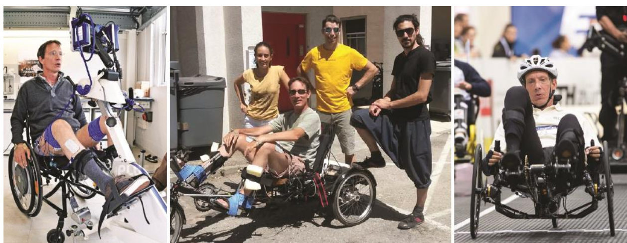
Fig 1. Training devices. Left: RT300 (Restorative Therapies, US); middle: HASE trike with Rehasstim 1 stimulator (Hasomed, Germany); Right: competing trike: Carbontrikes Race SL (Carbontrikes, Sweden) equipped with two Rehasstim 1 stimulators.
