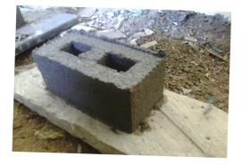
Figure 3: Freshly moulded hollow block
