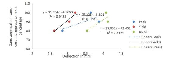
Figure 15: Aggregate mix ratio and deflection nexus
