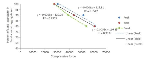
Figure 11: Aggregate mix ratio and compressive force nexus
