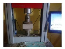
Figure 5: Masonry unit under compressive test
