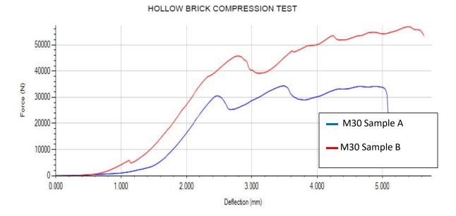
Figure 10: Stress strain curve for hollow block with 30% ceramic ware waste hollow block
