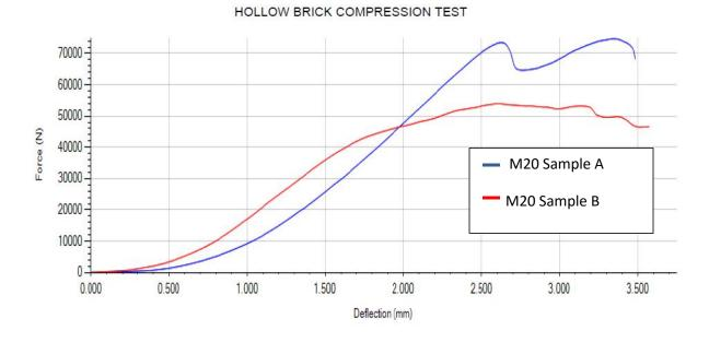
Figure 9: Stress strain curve for hollow block with 20% ceramic ware waste hollow block
