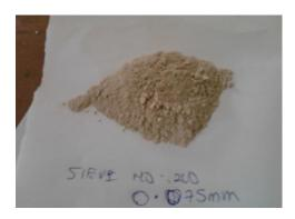
Figure 2: Granulated ceramic ware waste
