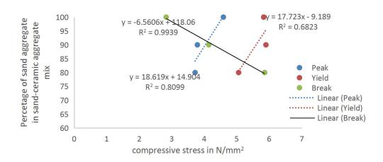
Figure 13: Aggregate mix ratio and compressive stress nexus
