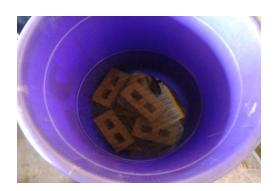
Figure 4: Hollow masonry unit under curing
