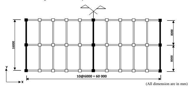
Figure 2: Plan of the Building Structural Model with Shear Walls
