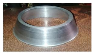
Figure 2.3: Mortar Flow Mould
