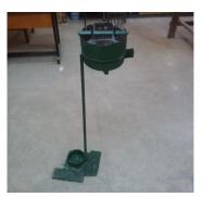
ACE456 were added to the paste and the flow time was determined for each increment.
