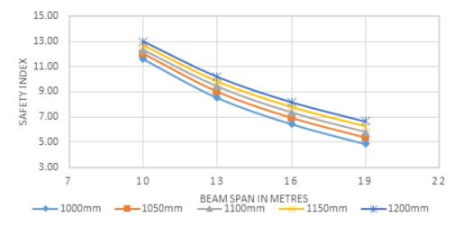
Figure 5: Flexural safety index Vs Beam span for various beam depth for 35 N/mm<sup>2</sup> characteristic strength of concrete
