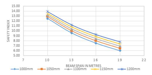
**Figure 6:** Flexural safety index Vs Beam span for various beam depth for 40 N/mm<sup>2</sup> characteristic strength of concrete
