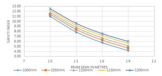
Figure 4: Flexural safety index Vs Beam span for various beam depth for 30 N/mm<sup>2</sup> characteristic strength of concrete
