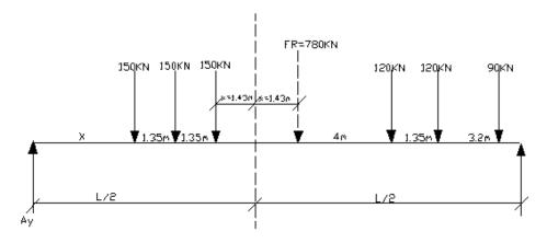
Figure 3: Arrangement of maximum bending of Load Model I
