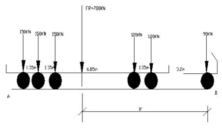
Figure 1: Load Distribution on 6-Axles (Sinotruck) according to Eurocode
