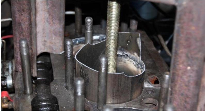
**Figure 4:** A Piston removal using sleeve puller
