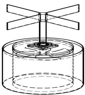
Figure 1: Exploded and Isometric Views of Cylindrical Wind Operated Evaporative Cooling Structure
