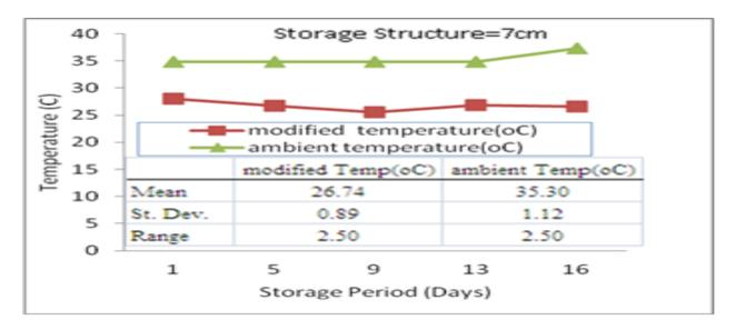
Figure 3: Variation in Temperature inside the Cooling Structures for Stored Tomatoes (Cylindrical Structure)
