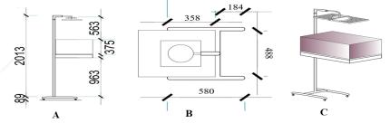
Figure 2: Isometric and orthographic views of the radiant warmer with measurements made in mm. A: Side view; B: Plan view and C: Isometric view.
