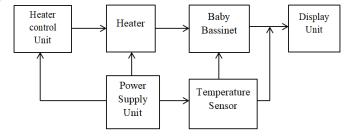
Figure I: System block diagram
