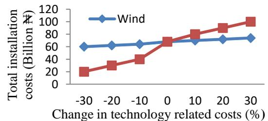
**Figure 2:** Sensitivity analysis of change in technology-related costs and total installation cost for on-grid arrangement.
