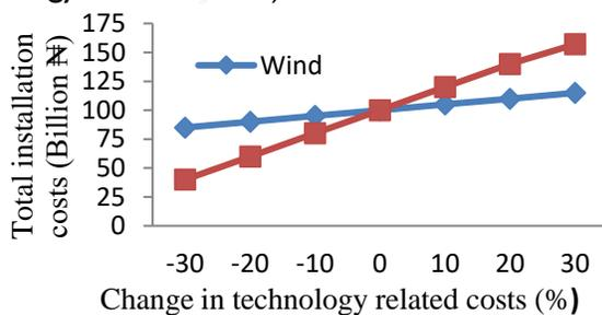
**Figure 1:** Sensitivity analysis of change in technology-related cost and total installation cost for off-grid arrangement.
