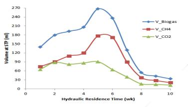
Figure 3: Biogas, methane and carbon dioxide production profiles based on CWCAM
