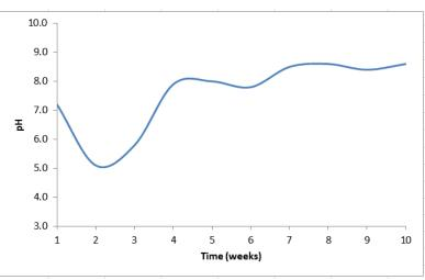
Figure 2: pH profiles of the digesting slurry
