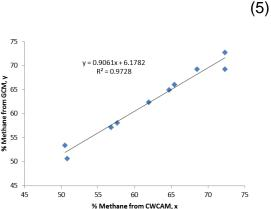
**Figure 5:** Comparisons between the GCM and CWCAM results for % methane determination.
