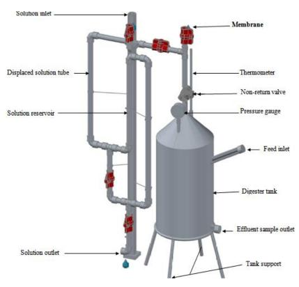
Figure 1: 15 | capacity digester system
