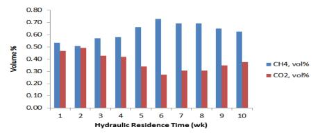
**Figure 4:** Methane and carbon dioxide contents in produced biogas (analysis based on CWCAM)
