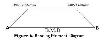
Maximum bending moment, M = 39852.6NmmSectional Modulus for square pipe or tube was assumed
