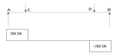
Figure 5. Shear Force Diagram
