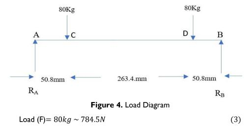
$R_A$  and  $R_B$  = vertical reaction at And B respectively.
