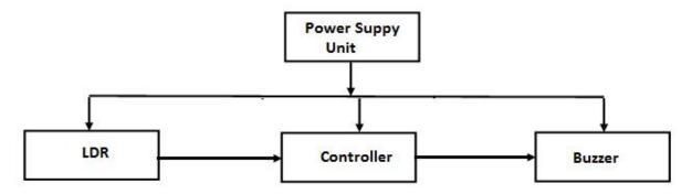
Figure 1: Block Diagram of an Arduino Based Alarm System.
