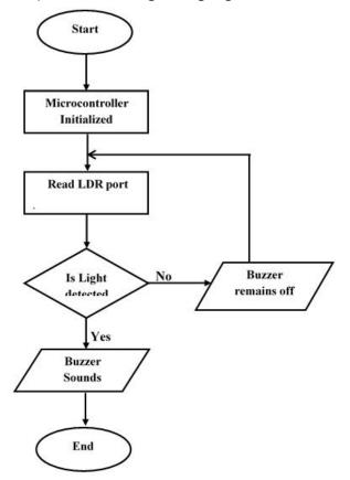
Figure 2: The System flowchart.
