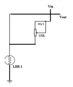
Figure 4: Voltage Divider between LDR and Potentiometer.
