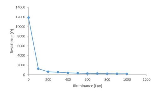
Figure 8: Result of plot for Resistance against Illuminance.
