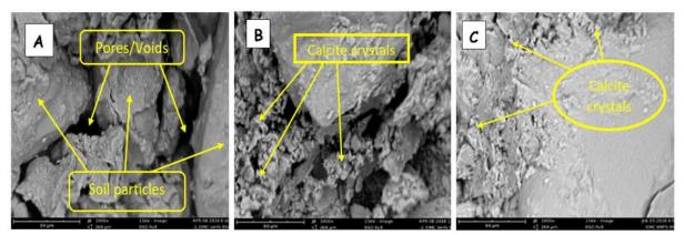
**Figure 7:** Micrograph at  $\times 1000$  Magnification: (A) natural soil, (B) Unsterilized soil treated with  $1.20 \times 10^{\circ}$  cells/ml suspension density at -2% OMC, (C) Sterilized soil treated with  $1.80 \times 10^{\circ}$  cells/ml suspension density at OMC
