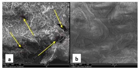
**Figure 8:** Micrograph at  $\times 1000$  Magnification of samples for Atterberg limits: (a) natural soil, (b) Unsterilized soil treated with  $1.20 \times 10^{9}$  cells/ml suspension density at -2% OMC
