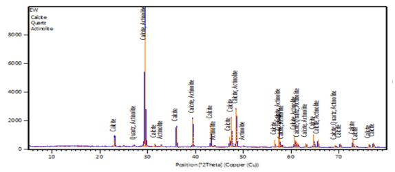
Figure I: X-ray Diffraction of precipitate obtained from test tube experiment
