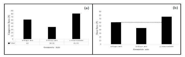
**Figure 3.** The compressive force **(a)** and shear force **(b)** test result for all three dimensions of the IT98K-573-1-1 cowpea. It was obtained from graphical plot on the computer screen of the UTM machine. It was the point of first failure of the plot.
