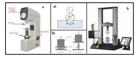
Figure 2. The Brinnel Hardness Tester is shown in (a) and the test demonstration (ai). The Universal Testing Machine (b) demonstrating test of a specimen (bi)
