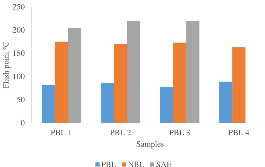
**Figure 5:** A chart of flash point for the biolubricant produced and SAE
