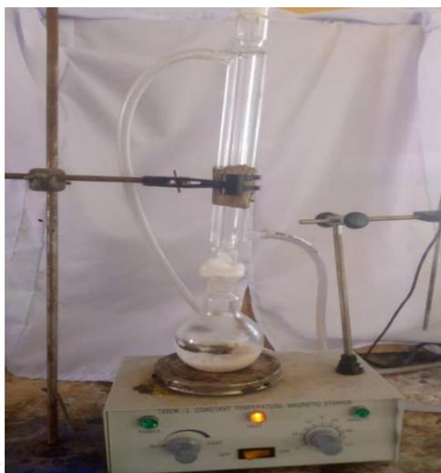
**Figure 3.** Transesterification set up
