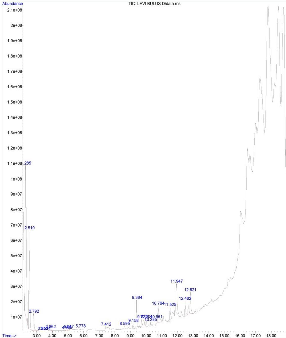
**Figure 6:** GCMS of fatty acid composition of parinari based lubricant
