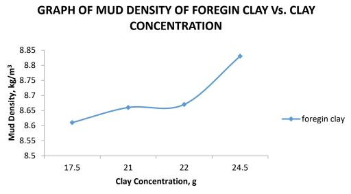
Figure 2: Foregin Clay Mud Density Vs. Clay Concentration.
