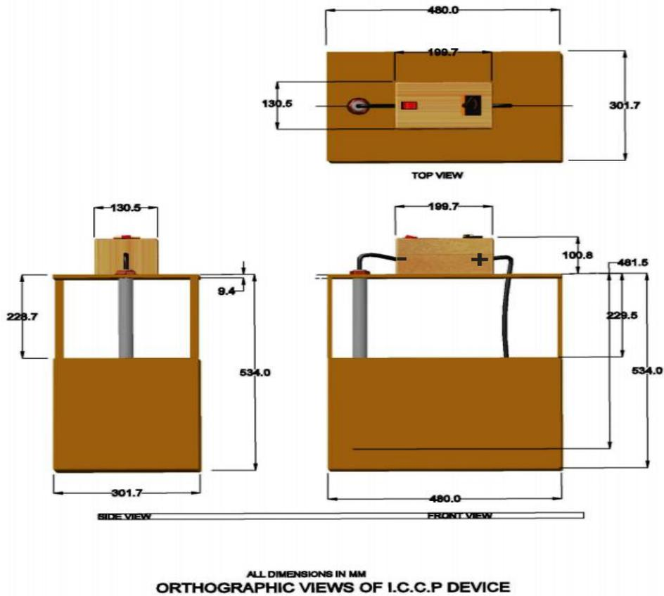
Figure 9a. 2D Orthographic projection of ICCP device
