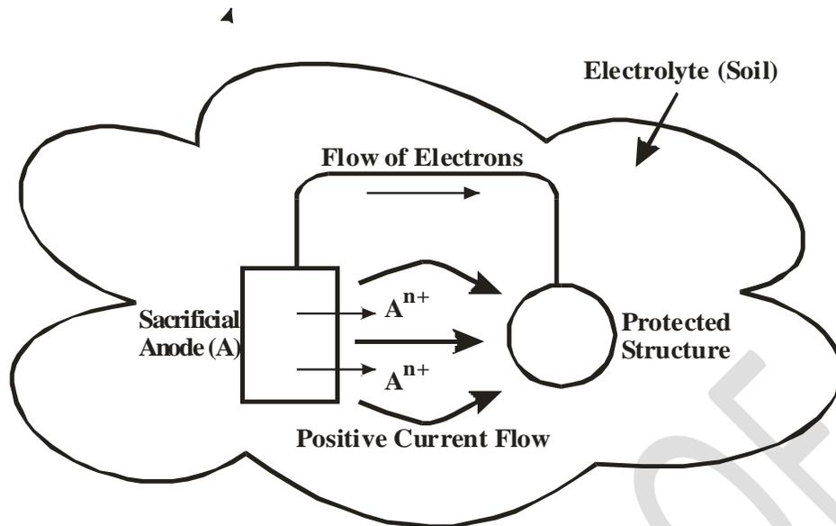
**Figure 1.** Schematic of Sacrificial Anode CP Method
