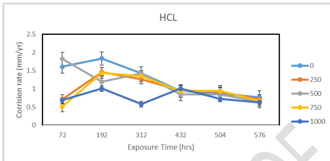
**Figure II:** Variation of Corrosion Rate (mm/yr) against Exposure Time (hr) of low carbon steel in 1 M HCl at different concentration of leaves extracts on cathodic impress device
