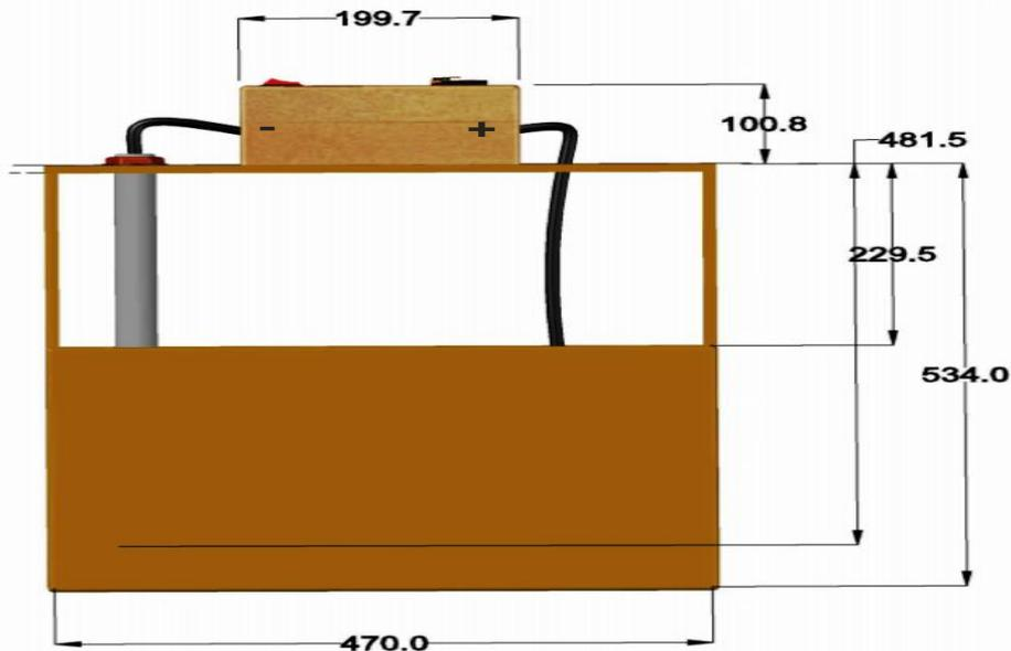
Figure 9b. 2D Orthographic projection of ICCP device front view. (All dimensions in mm)
