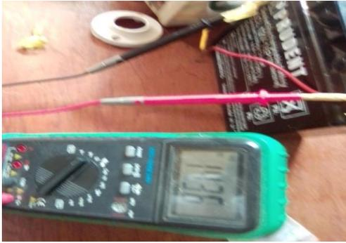
Figure 5: 14.36VDC battery voltage from digital meter with the proposed system
