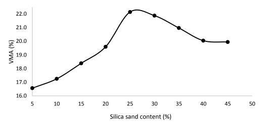
Figure 8: Variation of voids in mineral aggregate (VMA) with silica sand Content
