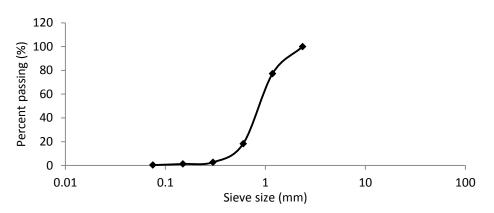
Figure 2: Particle size distribution curve for fine aggregate
