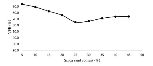
Figure 7: Variation of void filled with bitumen (VFB) with silica sand content
