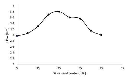
Figure 4: Variation of flow with silica sand content
