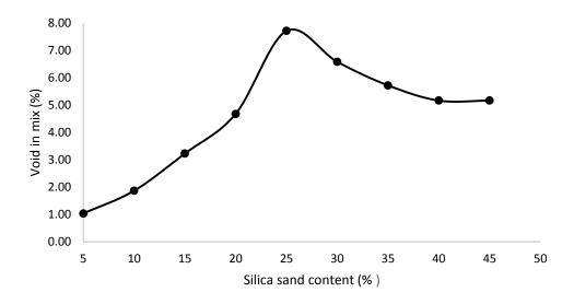
Figure 5: Variation of Void in the Mix (VIM) with silica sand content
