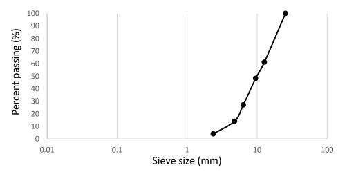
Figure 1: Particle size distribution curve for coarse aggregate
