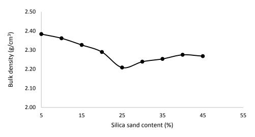
Figure 6: Variation of bulk density with silica sand content
