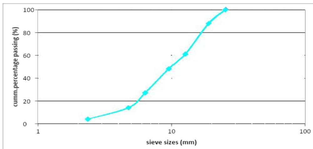
Figure 1: Sieve Analysis for Coarse Aggregate
