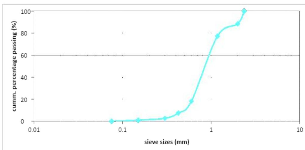
Figure 2: Sieve Analysis for Fine Aggregates
