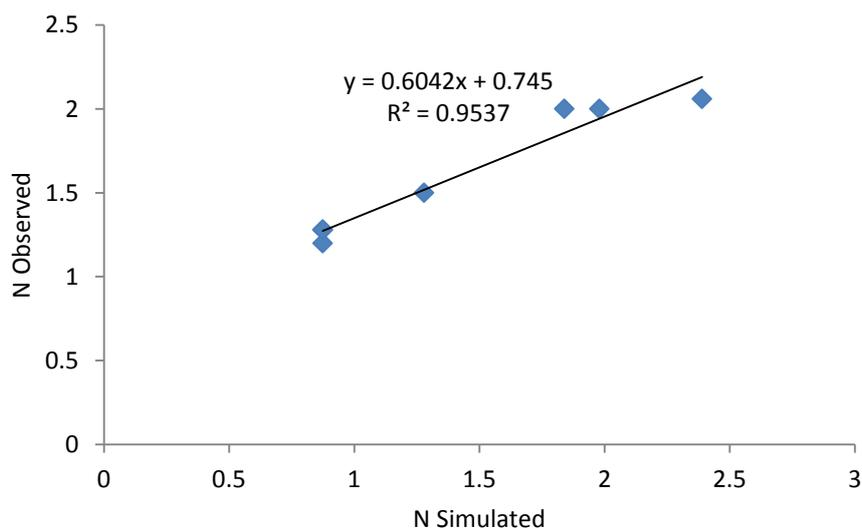
Figure 6: Correlation of observed and simulated removal of nitrogen in constructed wetland.
