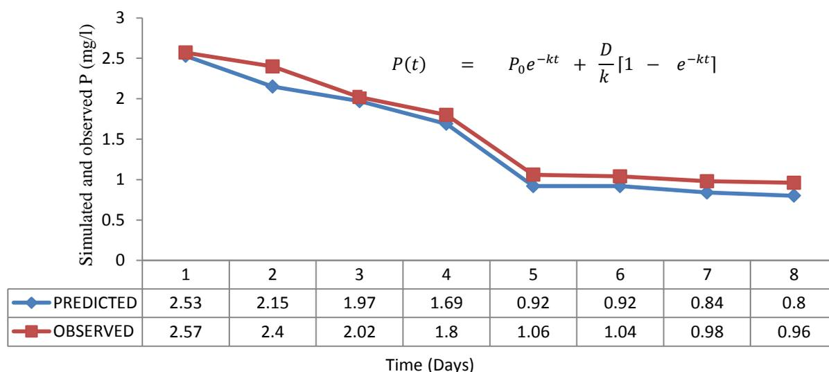
Figure 7: Simulated and observed variations for phosphorus removal in CW ( $P(t)$  = phosphorus concentration in wetland system (mg/l);  $P_0$  = initial concentration of phosphorus (mg/l);  $K$  = sum of phosphorus in wetland sinks (mg/l);  $D$  = rate of phosphorus input into the wetland ( $m^3/day$ );  $t$  = wetland retention time (d))
