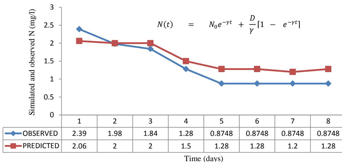
Figure 5: Simulated and observed variations for nitrogen removal in constructed wetland. ( $N(t)$  = nitrogen concentration in wetland system (mg/l);  $N_0$  = initial concentration of nitrogen (mg/l);  $\gamma$  = sum of nitrogen in wetland sinks (mg/l);  $D$  = rate of nitrogen input into the wetland ( $m^3/day$ ;  $t$  = wetland retention time (d))
