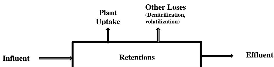
Figure 2: Conceptual model of nutrient removal in the constructed wetland (Udom et al., 2018)
