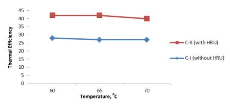
Figure 7: Overall thermal efficiencies at different operating conditions
