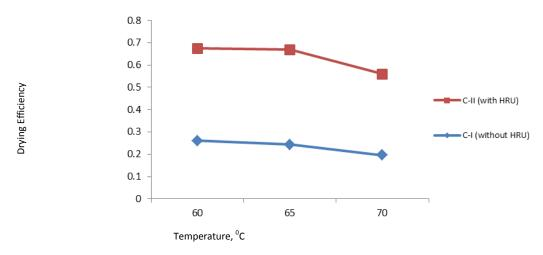
Figure 5: Drying efficiency at different operating conditions
