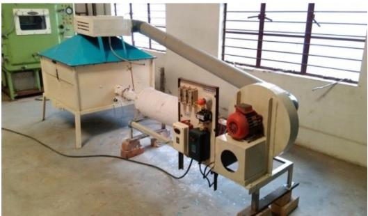
Figure 4:Flat-bed Dryer fitted with HRU
