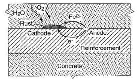
Figure I: Corrosion formation in concrete (Carino, 1999)
