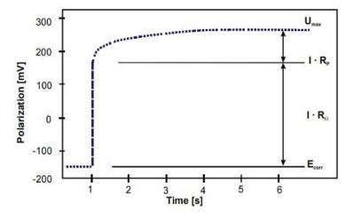
Figure 3: Electrochemical potential of steel against time (Sørensen and Frølund, 2002)
