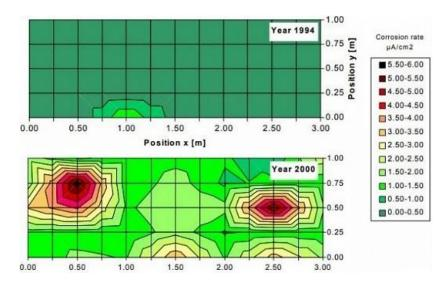
Figure 4: Corrosion rate using GPM over six years (Sørensen and Frølund, 2002)
