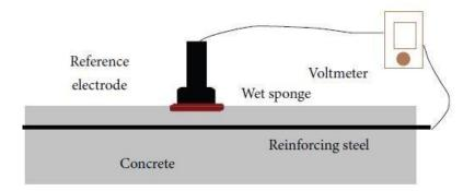
Figure 6: Typical half-cell potential set-up (Verma et al., 2014)
