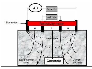
Figure 11: Wenner four-probe device measuring concrete resistivity (Carino, 1999)
