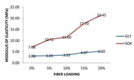
Figure 2: The effect of fibre loading on the Modulus of Elasticity of Corn-Plasticized Biocomposite.
