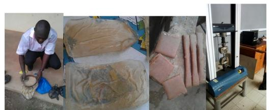
Figure I: (a) sieving of sawdust, (b) bioplastic, (c) test sample, (d) tensile test on machine
