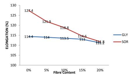
Figure 3: Effect of fiber content on elongation at break of biocomposite.
