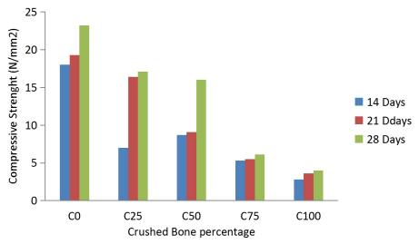
Figure 3: Variation of compressive strength with crushed bone percentage
