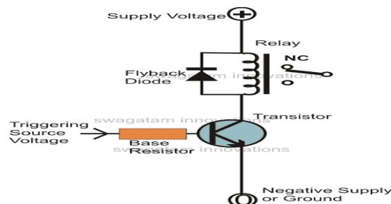
Figure 4: Basic Circuit Diagram of the relay driver
