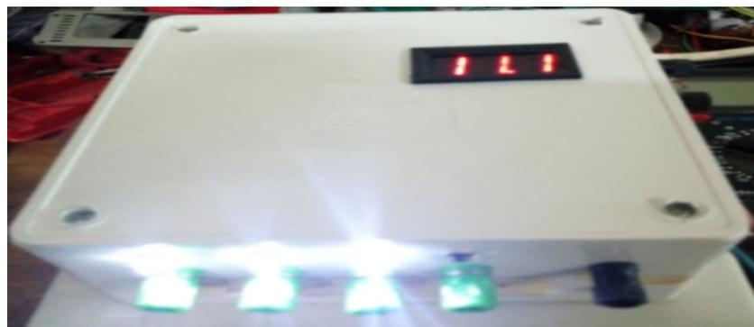
Figure 8: At 11.1V three outputs were active
