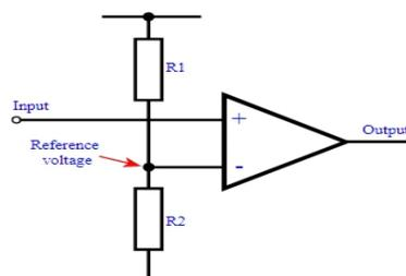
Figure 1: Circuit for a basic operational amplifier comparator
