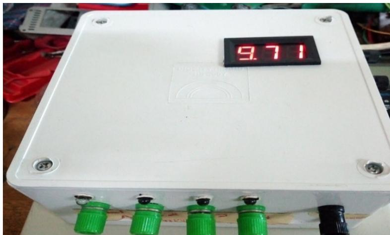
Figure 11: All outputs were inactive when the input voltage is below 10.0V
