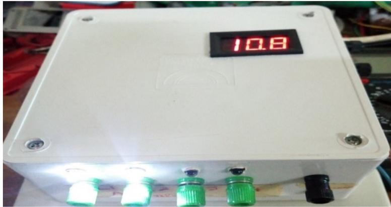
Figure 9: Two outputs were active when the input voltage is 10.8V.
