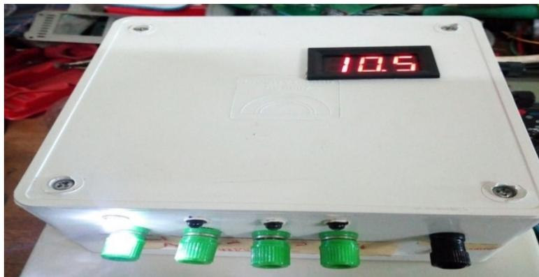
Figure 10: One output was active when the input voltage is 10.5V
