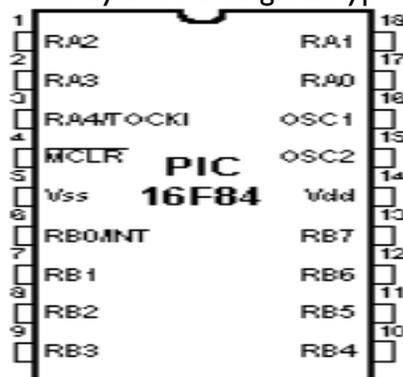
Figure 2: Pin assignment of PIC 16F84A
