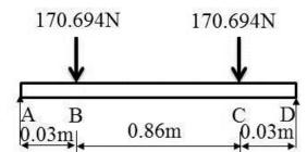
Figure 1: Loadings on the central shaft of drum
