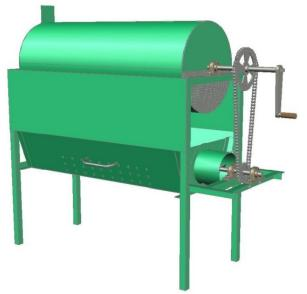
Figure 1. Isometric Views of the Roaster
