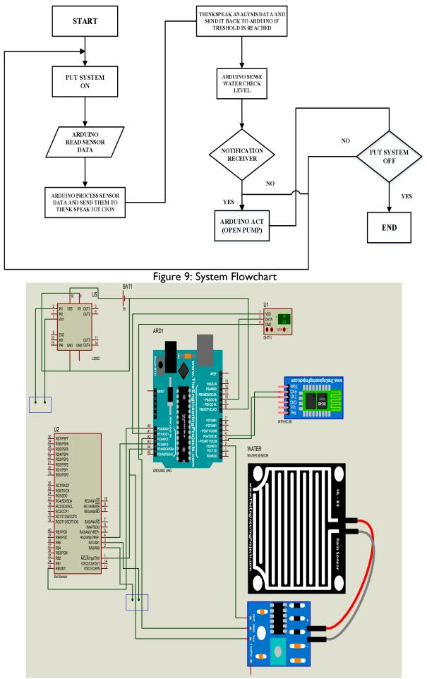
Figure 10: System Circuit Design
