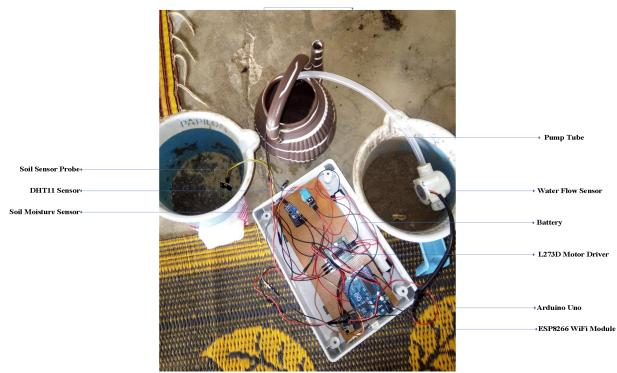
Figure 11: Prototype system
