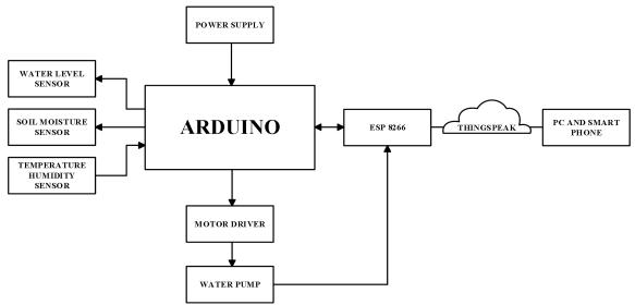
Figure I: Block diagram of an IoT based Irrigation System
