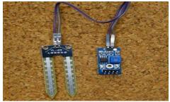
Figure 3: Soil moisture sensor
