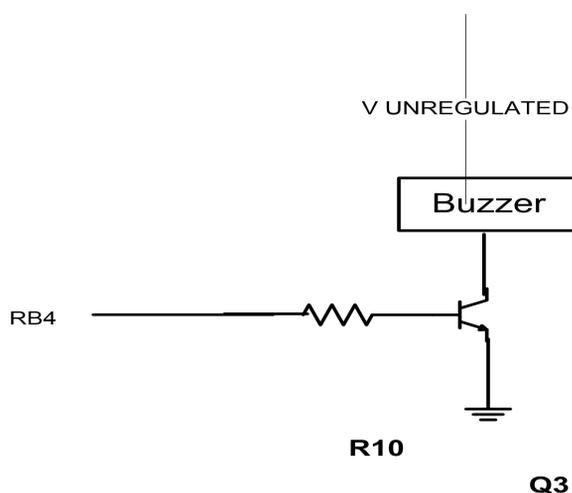
Figure 10: Buzzer interface circuit
