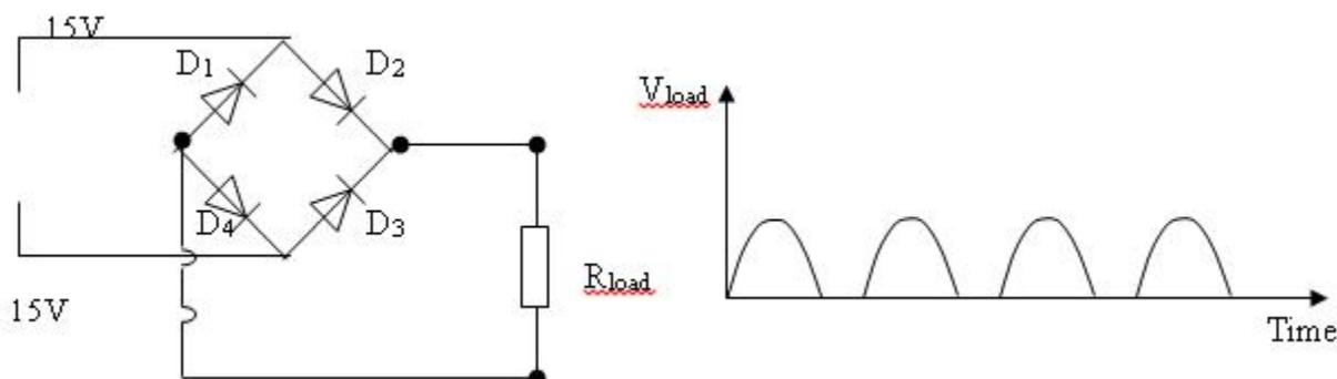
Figure 6: Circuit for Rectification and the Output Waveform
