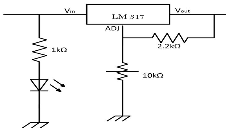
Figure 8: Voltage regulator circuit
