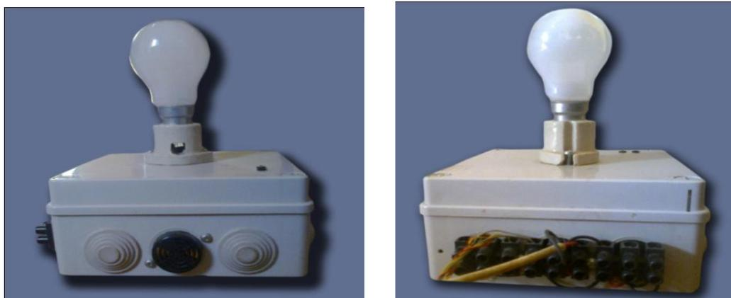
Figure 11: Front and Back view of the passive infrared automatic switching device
