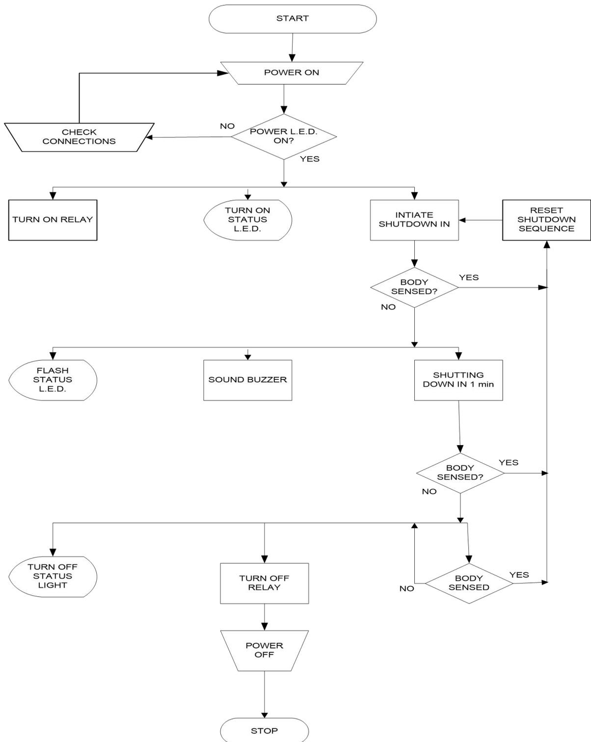
Figure 2: Process Flow Chart for Automatic switching system using PIR sensor
