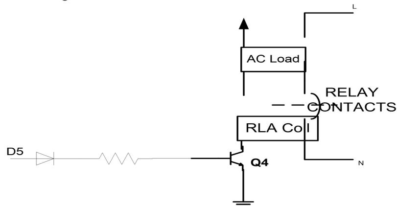
Figure 9: Relay interface circuit
