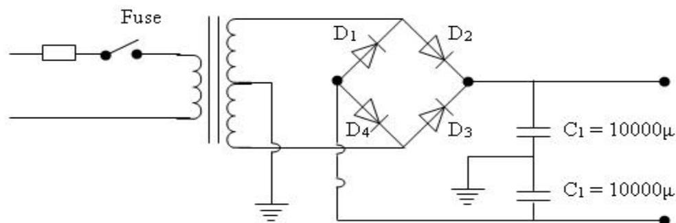
Figure 7: Power Supply Unit
