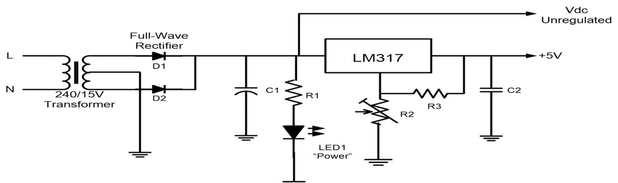
Figure 5: Power supply circuit
