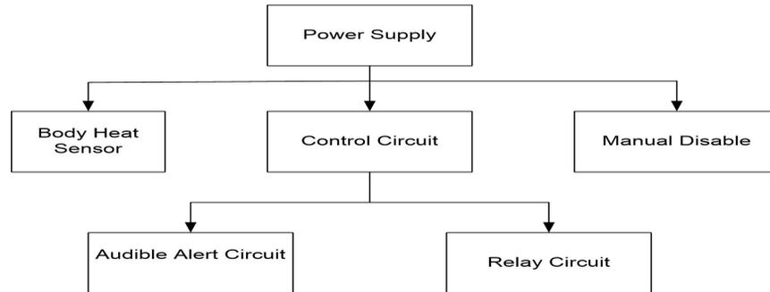
Figure 1: Block diagram of an Automatic switching system using PIR
