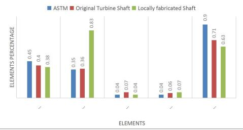
Figure 3: Comparison of elemental composition of ASTM standard, original turbine shaft and locally fabricated shaft.
