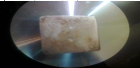
Figure I: Carbon Composition Test Sample of the Shaft
