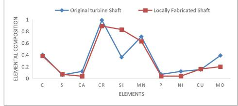
Figure 2: Comparison of elemental composition of original turbine shaft and locally fabricated shaft.
