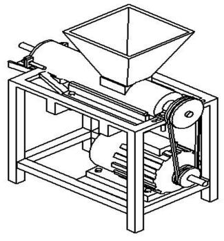
Figure 1: Isometric View of Fish Feed Pelletizing Machine
