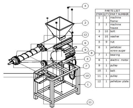
Figure 2: Exploded view Drawing of Fish Feed Palletizing Machine
