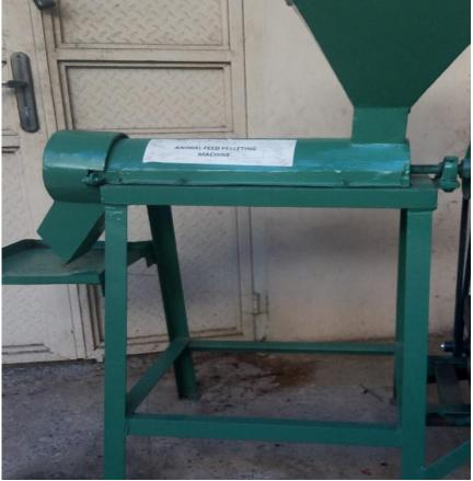
Figure 3: Modified Fish Feed Pelletizing Machine
