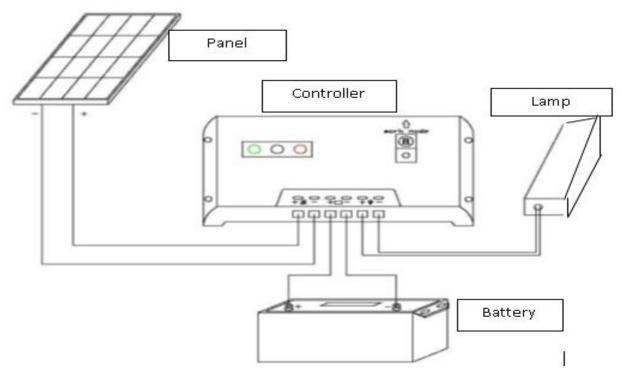
Figure 4: Installation diagram of the solar powered streetlight
