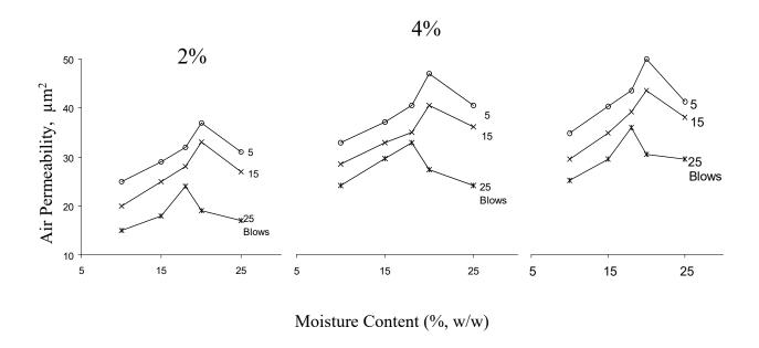
Figure 1: Air permeability vs moisture content for Ngala clay soil at different organic matter levels and proctor number of blows
