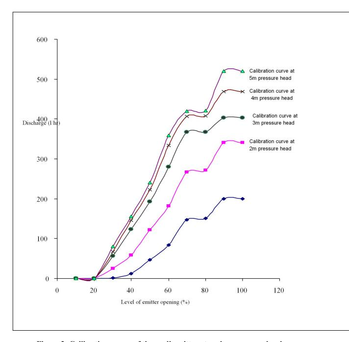
Figure 3: Calibration curves of the medi-emitter at various pressure heads
