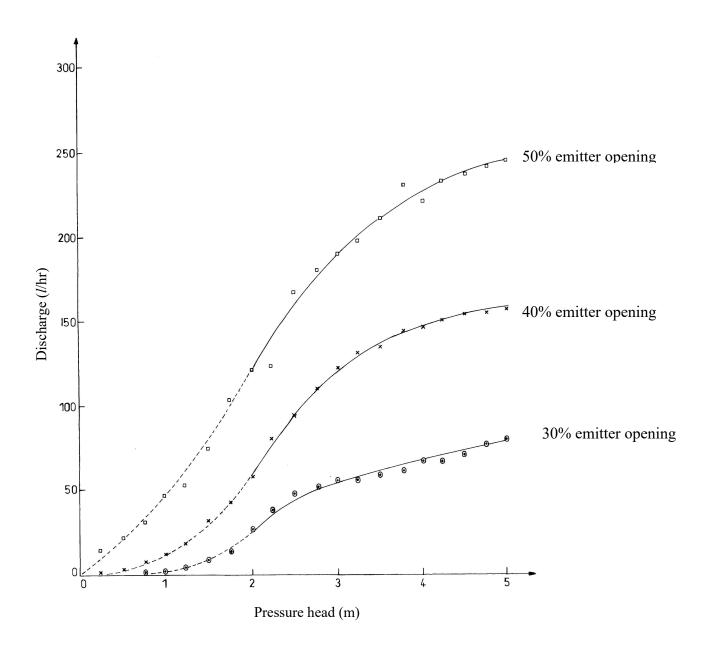
Figure 4: Emitter flow functions at 30 –50 % emitter opening
