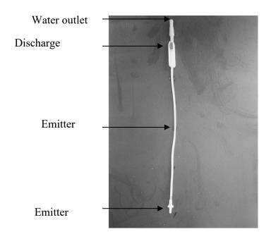
Figure 2: Main components of the medi-emitter
