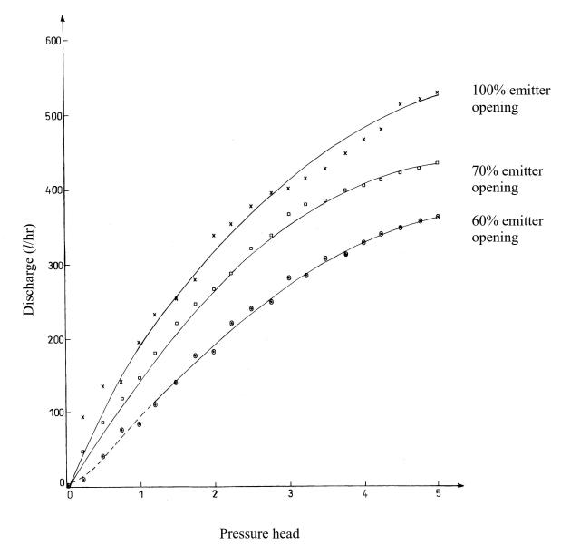
Figure 5: Emitter flow functions at 60 –100% emitter opening
