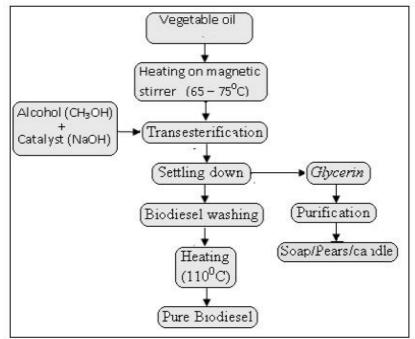
Figure I: Biodiesel production process flowchart (Jadhav et al. 2016)
