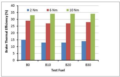
Figure 5: Brake Thermal Efficiency (BTE) of diesel and blends
