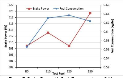
Figure 7: Brake Power Vs Fuel Consumption at 2 Nm
