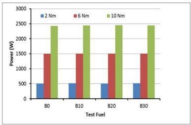
Figure 4: Brake Power of diesel and blends at different torques
