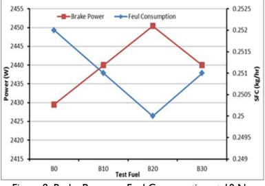
Figure 8: Brake Power vs Fuel Consumption at 10 Nm
