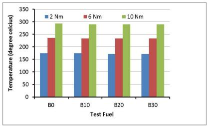
Figure 6: Exhaust temperature of diesel and blend
