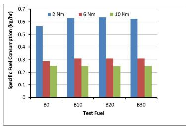
Figure 3: Specific fuel consumption of diesel and blends
