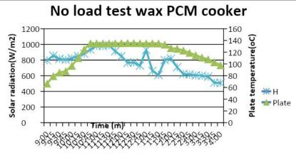
Figure 6: Thermal performance curve of plate temperature in SBC with Wax as TES in a test day
