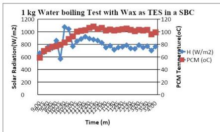
Figure 10: Full load test in a SBC showing PCM temperature behavior with corresponding solar radiation in a test day.
