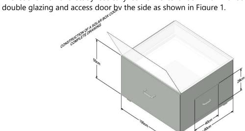
Figure 1: A double glazed Solar Box Cooker (SBC) with a booster mirror.
