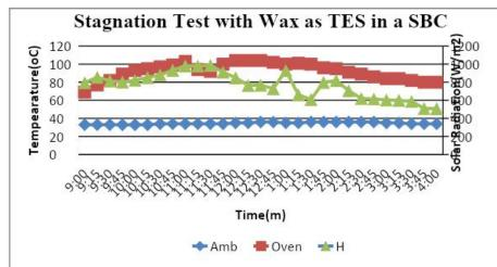
Figure 5: Thermal performance curve in an SBC with Wax as TES under no load condition in a test day showing ambient and oven temperature against corresponding solar radiation
