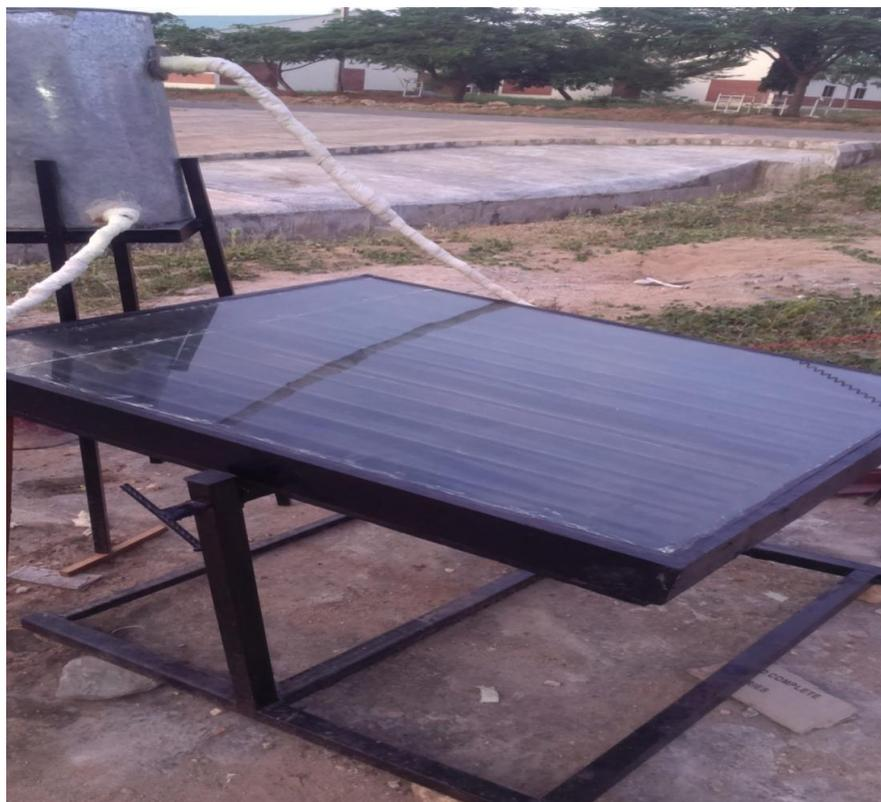
Figure 4: The Experimental setup of a solar water heater with PCM
