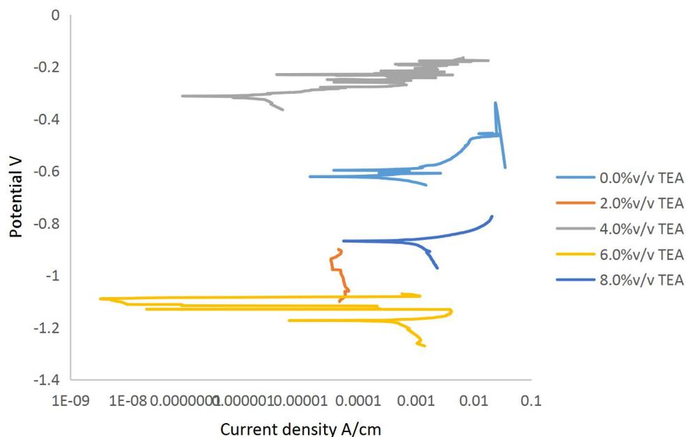
**Figure 2:** Potentiodynamic Polarization curves for multilayered mild steel/Al-Cr plates in 0.5M HCl solution and guava leaf extracts in absence and presence of different concentrations of triethylamine (TEA) as inoculant.
