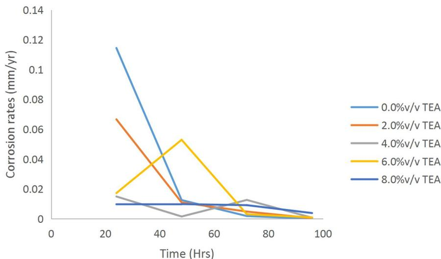
**Figure 1:** Variation of corrosion rates with time for different inoculant concentration.
