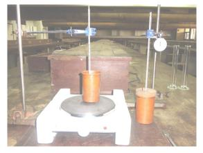
Figure 4. Set up for determination of thermal diffussivity of melon seeds
