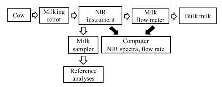
Figure 1. Flow chart of an on-line near-infrared spectroscopic sensing system for determining milk quality in an automatic milking system
