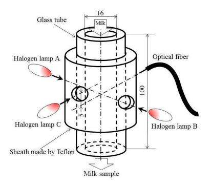
Figure 2. Schematic diagram of the optical system of milk chamber of the NIR spectrum sensor
